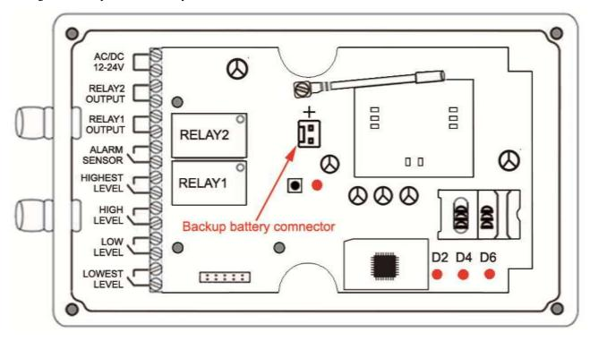
LED D2: SMS Receiver and Transmitter Status
