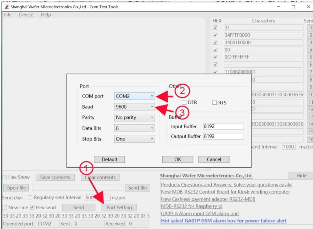
For example, if we need to do the Dex test, we need to select the Baud rate: 115200
