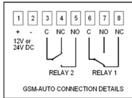
You must provide an external power source to the device you want to control. No voltage is present at the relay terminals (remember it is just a switch). The relay is normally connected in series with the positive (+) power wire of the device you want to control.
